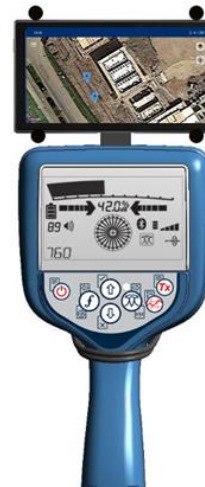
Figure 12.16: Phone/tablet correct position
