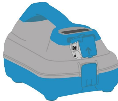
Figure 12.9: Transmitter DC Input
