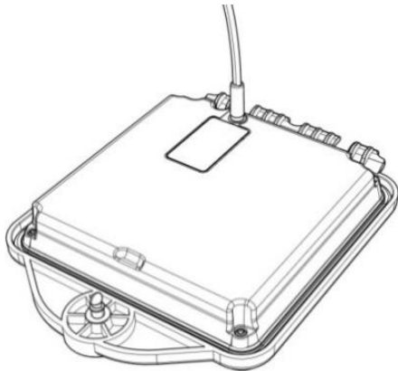
Figure 4.13 Charging the transmitter Li-ion battery pack
